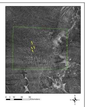
**Figure 2.** Magellan SAR data of Aglaonice dune field. The extent of the field is approximated with the green outline, and a small sampling of dune crestlines have been mapped in yellow.
