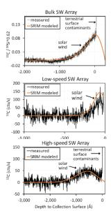
Fig. 2. <sup>12</sup>C profiles (black lines, background removed), from ion image data collected dur-SIMS back-side ing depth profiling Genesis collectors. Scaled SRIM models (thick orange lines) are overlain for reference. The Si break through points are at 0 Å. Note: the y-axis scale for the bulk measurement includes a gamma correction.
