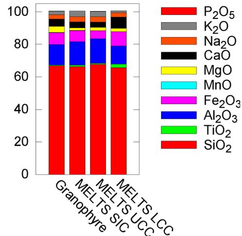
**Fig. 1:** MELTS model results. Input data for SIC from [11], UCC from [12], LCC from [13]. Granophyre composition determined by XRF analysis.
