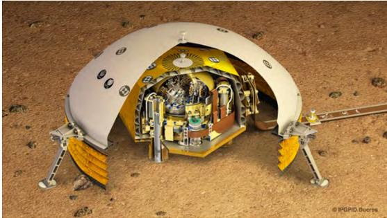
Figure 4: Final configuration of SEIS with the three layers of thermal protection of the VBBs (Evacuated Sphere, Thermal Blanket and Wind Shield). The two last are also shielding the SPs.
