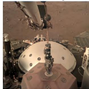
Figure 1: On-deck configuration with the grapple connected to SEIS. SEIS is in front, with the white Wind and Thermal Shield behind.
