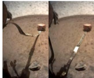
Figure 2: SEIS on the ground before tether release (left) and after tether release (right).
