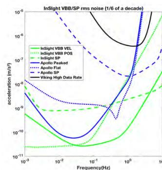
Figure 2: RMS self-noise of the three main outputs of the SEIS instrument (VBB VEL, VBB POS and SP VEL), in acceleration for a 1/6 decade bandwidth, as a function of the central frequency of the bandwidth. This is compared to the Apollo and Viking resolution (Least Significant Bit).
