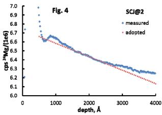
product of the RSF and the (implant Al)/Mg depth integral [1]; this assumes that the charging variations in the Al/Mg counting rate ratios cancel. With one exception, constant Al/Mg ratios are observed after sputtering through the SCJ implants or beyond transients in the unimplanted SC3 profiles. The exception, profile SCJ@5 is also much broader and appears to have much larger amounts of charging.
