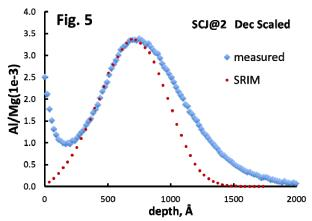
estimated precision of a single analysis is 4.8%. The measured fluence standard deviation is higher, 6.0%, which we adopt as the precision of the SCJ fluence, giving  $4.67\pm0.30x10^{14}/cm^2$  as the calibrated fluence of the SCJ implant where the quoted error also includes a 2.2% contribution from the error in the RSF. The measured fluence is within 1  $\sigma$  of the nominal  $5x10^{14}$  atoms/cm<sup>2</sup>.
