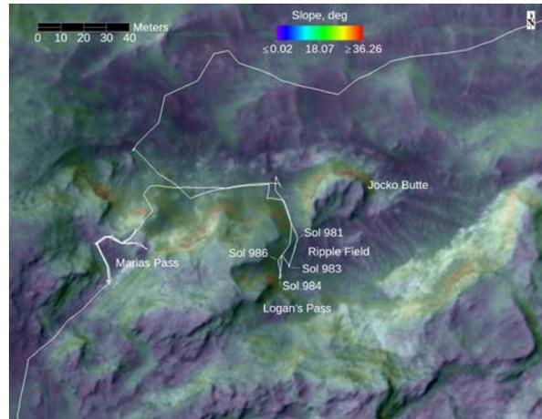
**Figure 4:** Portion of a HiRISE mosaic overlain with rover-scale slopes for Curiosity's traverses toward Logan's Pass and in Marias Pass. The rover was commanded to start a northerly route on sol 986, which led to successful traverses through Marias Pass.
