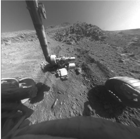
**Figure 2:** Front Hazcam image acquired on sol 4313 after Opportunity backed down after an unsuccessful sol 4311 uphill drive to the outcrop known as Whitehouse. Note the deep wheel tracks generated during the uphill drive attempt.
