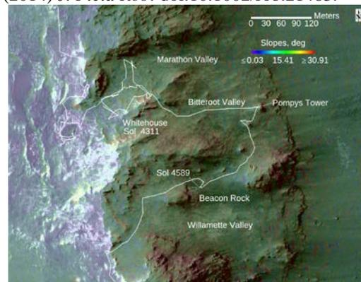
**Figure 1:** Portion of a HiRISE mosaic overlain with rover-scale slopes and Opportunity's traverses for a portion of Cape Tribulation. Mobility difficulties were encountered while attempting uphill drives to Whitehouse and Beacon Rock.
