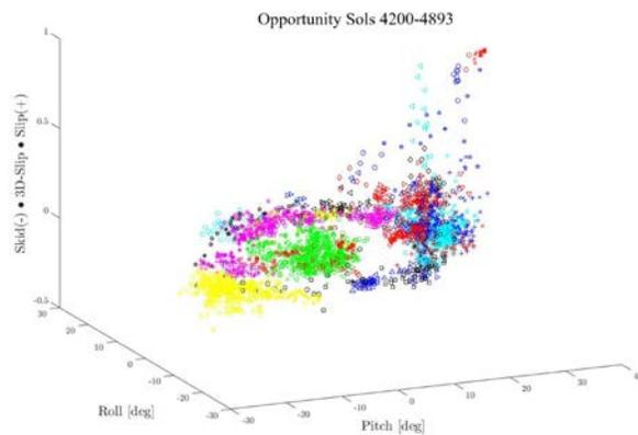
**Figure 3:** Plot of slip/skid as a function of pitch and roll for a wide range of Opportunity's drives on Cape Tribulation. High slip values are associated with high pitch values traversing uphill whereas high skid values are associated with steep descents. Each color/pattern is for a specific drive. Skid and slip are derived using visual odometry [4]. Slip occurs when the 3D distance is less than commanded and skid when it is more than commanded.
