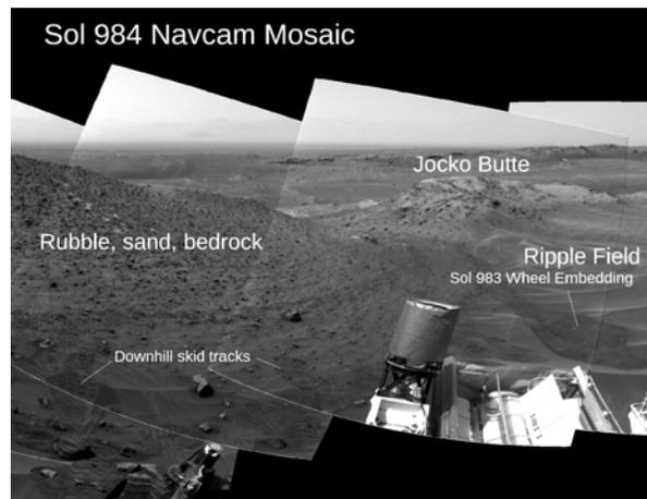
**Figure 5:** Portion of a Curiosity Navcam mosaic looking back at the rover left front wheel embedding in ripple sand that caused termination of the sol 983 drive, together with the wheel tracks showing skid during the aborted sol 984 drive on the rubble, sand, and bedrock-dominated slope.
