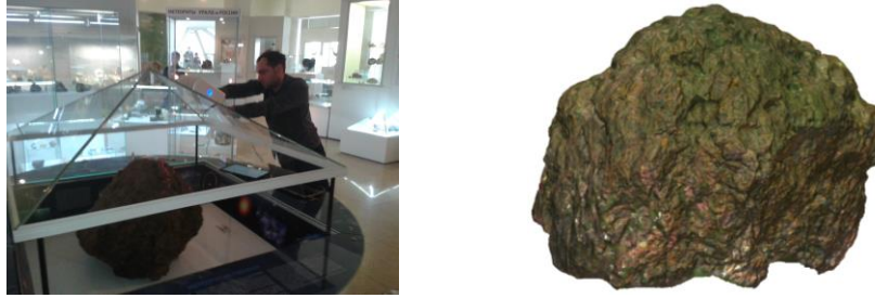
Fig. 1. 3D laser scanning of the 502 kg Chelyabinsk meteorite (left) and resulting 3D model (right).
