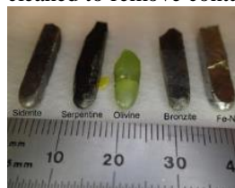
Figure 1: Set of pins used in the adhesion testing.
