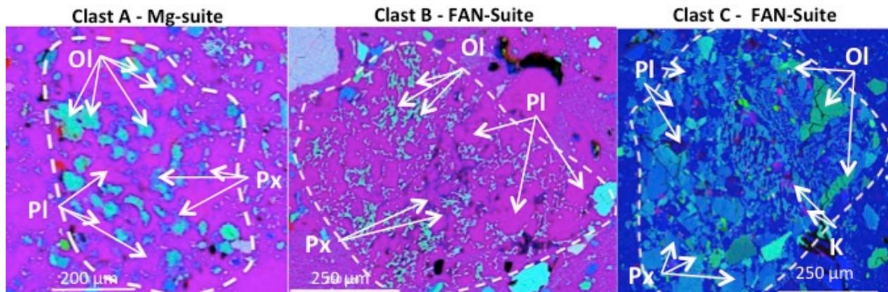
**Figure 3:** Combined element maps of clasts from NWA 10986. Element maps for Clast A and B are Si K $\alpha$ , Fe K $\alpha$ , and Ca K $\alpha$ . The element map for Clast C is Si K $\alpha$ , Fe K $\alpha$ , and K K $\alpha$ . Pink areas within Clast C indicate high-K.
