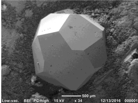
**Figure 2:** SEM image of euhedral analcime crystallized on the fracture surface of an impact melt-bearing breccia located ~1300 mbsf (sample 293-1-8-10.) Scale bar is 500 $\mu$ m wide.
