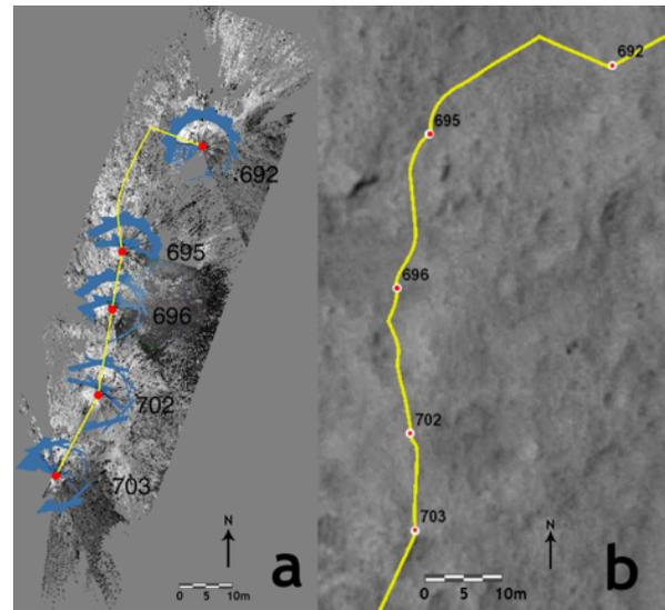
**Fig. 3** (a) Reconstructed traverse path (yellow) of Curiosity as determined using Agisoft Photoscan Professional and Navcam images from sols 692, 695, 696, 702, and 703. Red points show estimated rover position on these sols and blue polygons denote estimated camera poses. (b) Actual traverse map for Curiosity for sols 692-703 [5].
