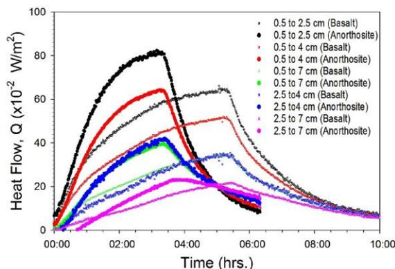
Figure 3: Comparison of heat flow profile during heating for Basalt and Anorthosite samples
