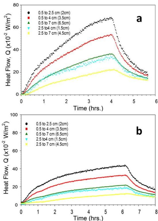
Figure 2: Comparison of heat flow with (a) Sample cup without perforations (b) Sample Cup with perforations
