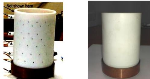
Figure 1: Designed Sample holders with and without perforations.
