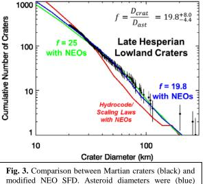
modified NEO SFD. Asteroid diameters were (blue) multiplied by f = 19.8, (green) f = 25, and (red) input into a crater scaling law designed to match hydrocode results.
