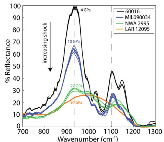
**Figure 2:** FTIR reflectance spectra for a select range of plagioclase crystals within different planetary materials (Moon and Mars), illustrating the differences in reflectance spectra with increasing shock pressure. Increasing shock is evidenced by a general smoothing of spectrum (e.g. in martian meteorite LAR 12095, which contains extremely shocked ‘maskelynitised’ mineral).
