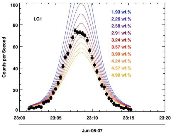
**Figure 1.** Neutron count rates, measured by the MESSENGER NS (from “LG1” detector) during the V2 flyby. Measured values and one-standard-deviation statistical errors are shown in black. Neutron models are shown as colored lines, with each color representing a different  $N_2$  concentration. LG1 was the NS sensor most sensitive to thermal neutrons during V2.
