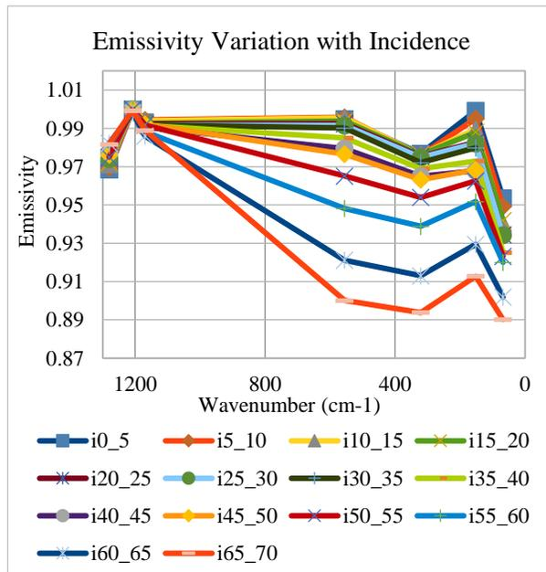
**Figure 1.** The emissivity spectra measured at varying incidence angles from a spot within Mare Tranquilitatis. Note the decrease in spectral signal with increasing incidence angle.
