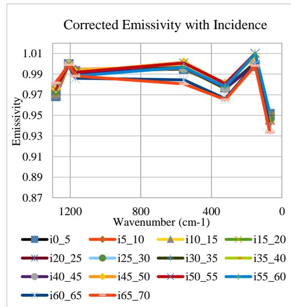
**Figure 3.** The emissivity spectra corrected with the calibration function. While there is still variability in the spectra with incidence, the signal is increased and there is more consistency to the data.
