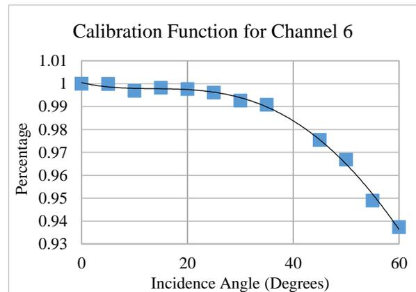
**Figure 2.** The calibration function for our correction is derived by dividing each emissivity value by the 0° incidence angle emissivity for each channel.
