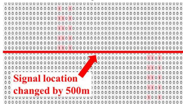
Fig.3: A part of output obtained in function test of dust count mode. The output of 50bins for a shot is listed in one line and the series of results are shown line by line. An output of 1 (over the threshold) is represented by hatched pink.
