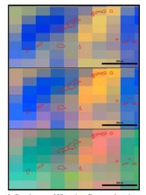
**Figure 4.** Southeast of Huggins Crater, showing spectral slopes indicative of steep terrain [8]. From top to bottom: DCS 875, 964, and 642 basemaps, with RSL outlines (red).
