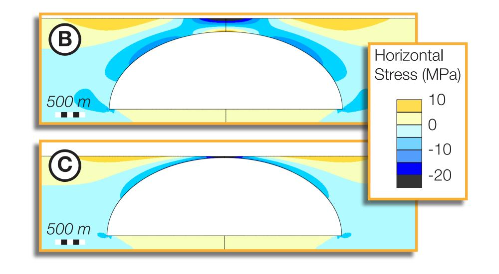
We are still exploring **regional tectonic stresses** and **cooling and contraction** of the lava tube. The modes of failure shown here, however, indicate that extensional far-field stresses may allow larger or thinner-roofed tubes.
