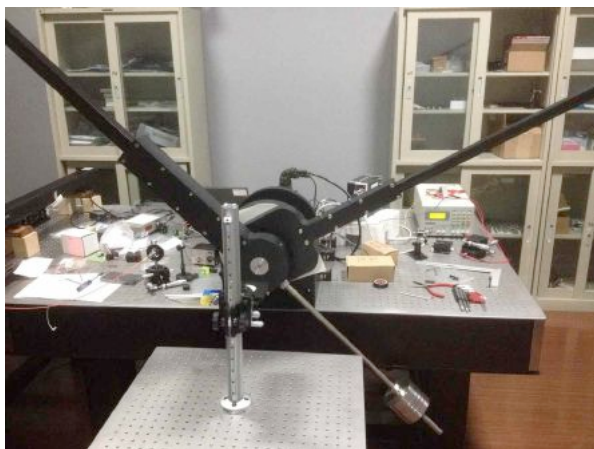
Fig. 2. The goniometric system with the sample holder in the front.
