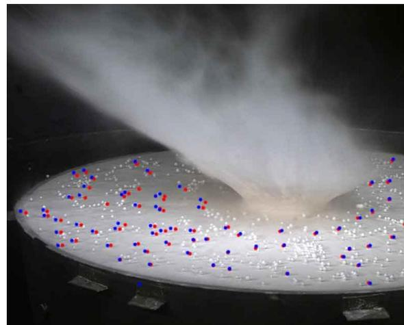
Figure 3 - Laboratory experiment of a 0.25 inch Pyrex projectile impacting dolomite at 45° (from the right) and approximately 5 km/s. Red dots indicate the initial position of some of the Styrofoam pearl tracers. Blue dots indicate the position of the tracers at 1935  $\mu$ s into the impact. Impact vapor expansion interacting with the ambient atmosphere mobilizes the tracers to meter per second velocities.
