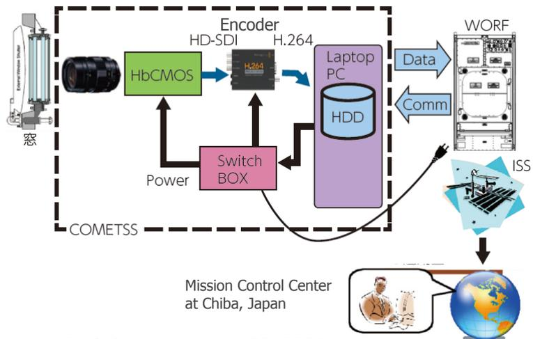
Fig. 3. Block diagram of the COMETSS system
