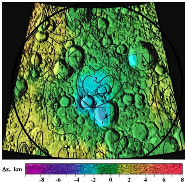
**Figure 1.** Radial field strength in nT at ~ 25 km altitude measured by the LP magnetometer over the Coulomb-Sarton basin. The contour interval is 0.2 nT.
