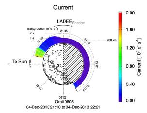
**Figure 2:** An example of current measurements taken by the LADEE LDEX instrument for orbit 605 on December 4, 2013. The observation begins at approximately 21:09 with elevated, temporally variable levels of current before diminishing near 21:15.
