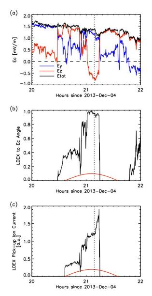
Figure 3: (a) The convection electric field components (colored lines) and magnitude (black line) as measured by the ARTEMIS spacecraft. (b) The cosine of the angle between the convection electric field and the LDEX instrument boresight. (c) The model-predicted pick-up ion current into the LDEX instrument in arbitrary units for approximately one orbit on December 4, 2013. The red semi-circle denotes the period when LADEE/LDEX was on the lunar dayside.
