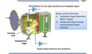
**Figure 1.** The schematic drawing of LDEX. Dust particles enter the detector through a triplet of transparent grids that prevent solar wind electrons flooding the instrument.
