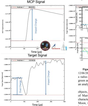
**Figure 3.** Impact waveforms recorded by LDEX at the Colorado dust accelerator of an iron particle with a radius of 1.06  $\mu$ m and speed of 1.89 km/s. The waveforms are recorded (50 samples with a dt of 8  $\mu$ s) and transmitted to ground. At the accelerator the dust particles are highly charged and the target signal also shows the effect of their 'image' charge on the target.
