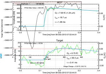
**Figure 4.** Impact recorded in orbit around the Moon on 12/06/2013. Based on preliminary analysis, this particle had a radius of ~1.2 µm, and carried a charge of ~2.5 fC. The green and blue lines show the recorded waveforms and an analytical fit, respectively.
