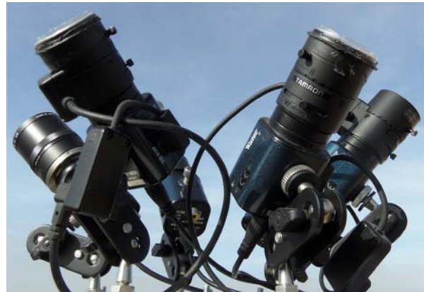
Figure 1. One of the new 6-videospectrographs arrays employed at the Cerro Negro mobile station.
