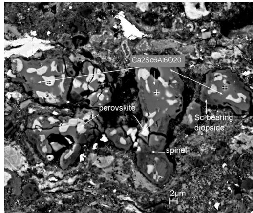
**Fig. 1.** Backscatter electron (BSE) image showing  $\text{Ca}_2\text{Sc}_6\text{Al}_6\text{O}_{20}$  associated with perovskite, spinel and diopside in a CAI from Murchison. SIMS spots are indicated with cross.
