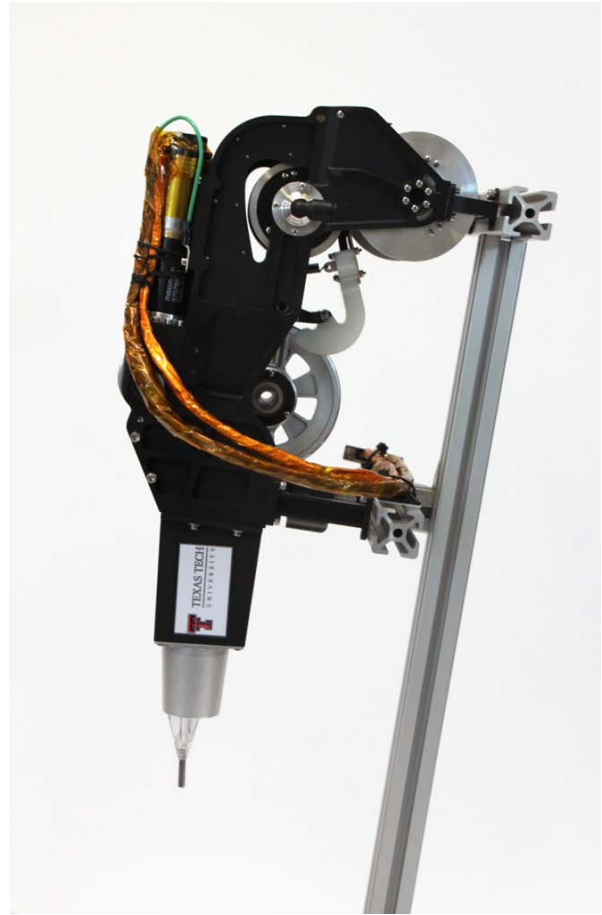
Figure 3: A photograph of the latest prototype of the heat flow system in a stowed configuration.
