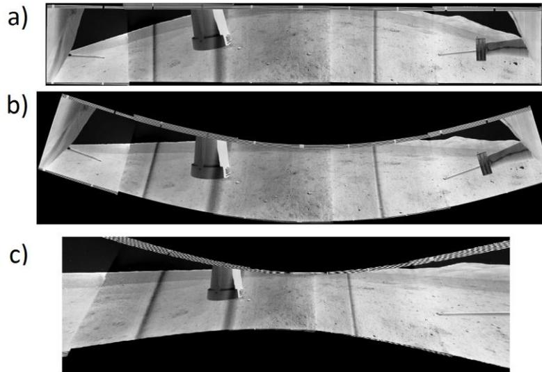
Fig. 1. Lunokhod-2 panorama a) assembled from archive fragments (spherical projection); b) assembled and brought to the horizon (spherical projection); c) assembled, brought to the horizon, and transformed into central projection
