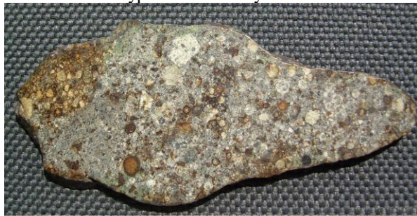
Fig. 1. Optical image of NWA 4560 meteorite. Chondrules and matrix are seen. Olivine crystals are yellowish and rusty, pyroxene crystals are greenish and blackish (augite), and plagioclase are white.
