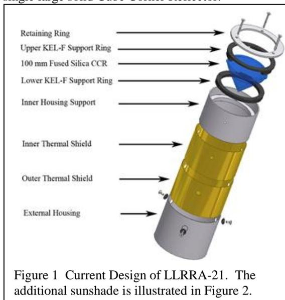
Figure 1 Current Design of LLRRA-21. The additional sunshade is illustrated in Figure 2.
