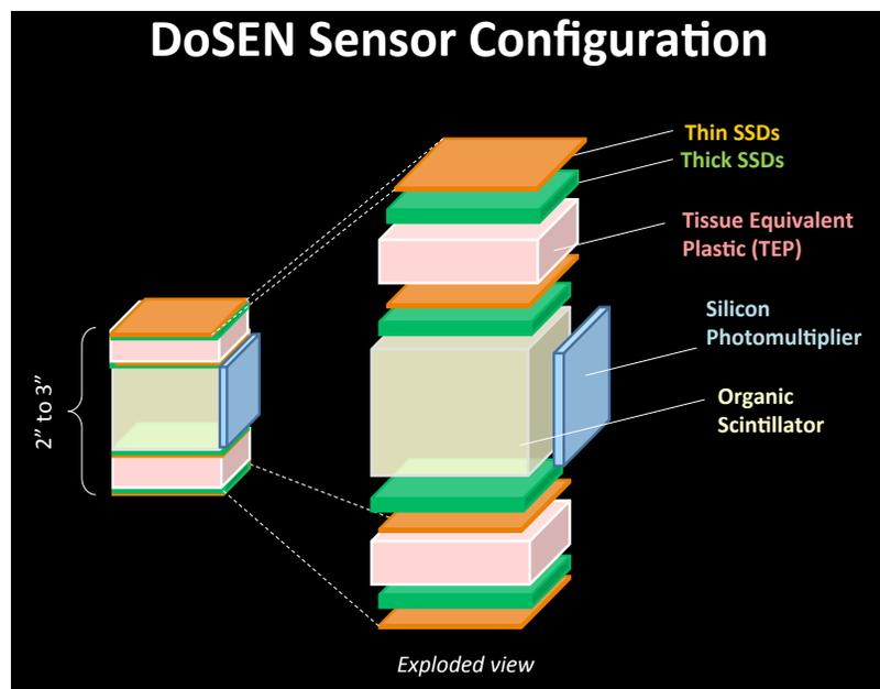
**Figure 1.** The DoSEN sensor configuration includes a combination of Solid State Detectors (SSDs), organic scintillator with PSD and Si photomultipliers (SiPMs) allowing coincident detection of energetic particle LET and neutrons. The unique coincidence offered by LET & neutron detection promises a significant advance for a new generation of dosimetry measurements.
