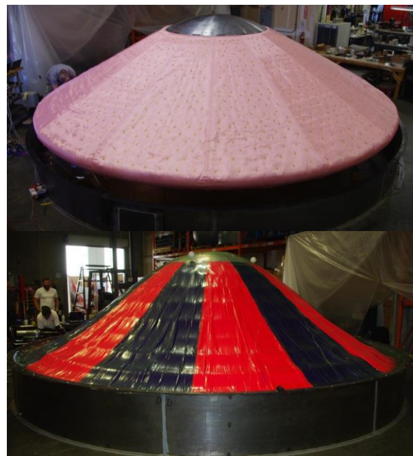
Figure 2. 6m HIAD with TPS (top), under 50,000 lbs of static load (bottom)
