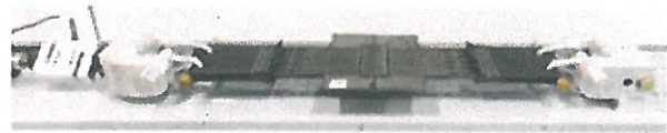
Fig 1. Photograph of arcjet test article with seam joining two pieces of carbon fabric during load conditioning.
