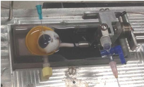
**Figure 1:** Photograph of a porcine eye being prepared for testing. The meninges (optic nerve sheath) and the eye itself have both been cannulated, using the silver fitting (middle of the photo) and the blue needle (entering anterior chamber), respectively.
