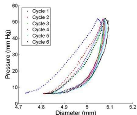
**Figure 2:** Pressure-diameter curves for a single porcine meninges, tested over six 7-50 mmHg pressure cycles. This information, together with the geometry of the meninges, allows determination of the tangent modulus (stiffness).
