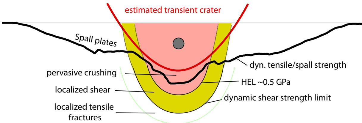
**Fig. 1:** Schematic overview of deformation in a sandstone target impacted by a 1 cm steel projectile (center) at 4.5 km/s. Subsurface damage was mapped in [10], final crater profile and transient crater are from [7]. Most of the transient crater is dominated by material damaged above the Hugoniot elastic limit, and thus may not show strain rate or Weibull effects seen for spallation.
