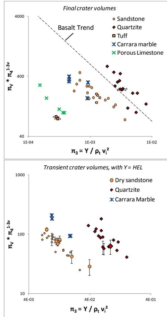
**Fig. 2:** Scaling of final craters (top), using quasi-static UCS values for  $Y$ , and scaling of transient craters (bottom) using the Hugoniot elastic limit (HEL values from [13]). Both plots are problematic, as discussed in the text.
