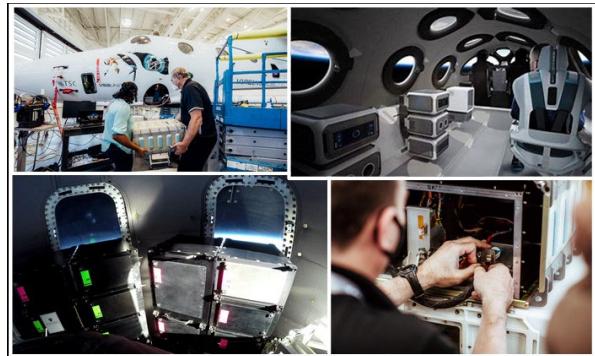
Figure 2. Integrations of payloads on commercial suborbital spacecraft.
