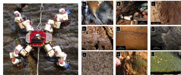
Figure 1: LEMUR III demonstrates rock-climbing capabilities to better detect biopatterns.
