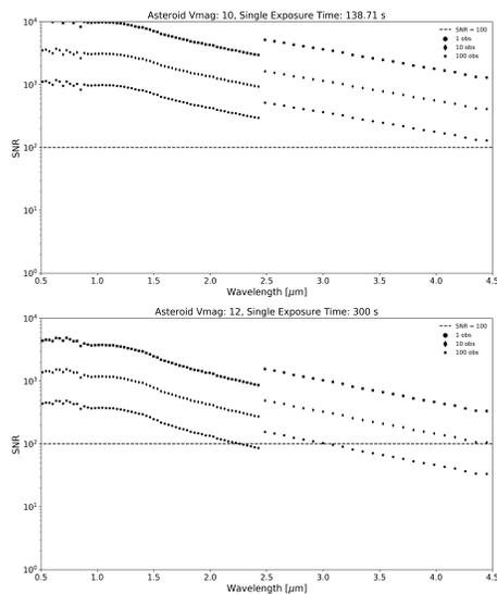
Figure 2: SNR achieved in each spectral band for observations of an asteroid with a visible magnitude of 10 (top) and 12 (bottom) with Twinkle over 1, 10 and 100 observations.
