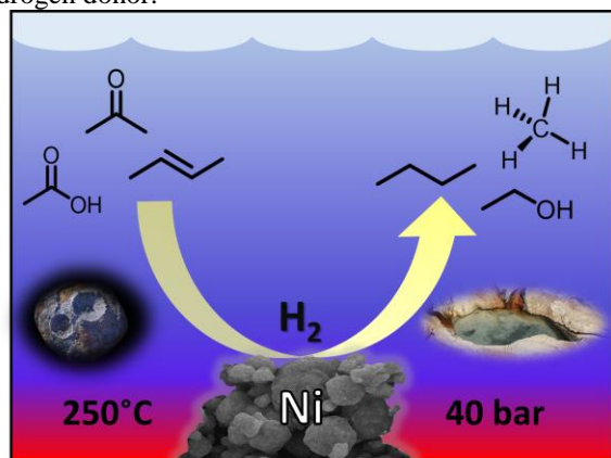
Figure 1. Schematic representation of organic functional group transformations observed under hydrothermal conditions, catalyzed by crystalline metallic nickel.
