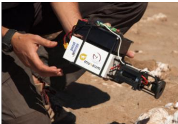
Figure 1. Our LIBS instrument is a handheld unit that can perform identification/quantification of virtually all elements and some molecular species (CN, CH, CC). Relevant applications: elemental ID, mineralogy, scouting, and exploration.
