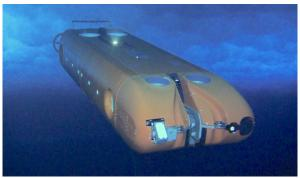
**Deployment:** ARTEMIS was deployed to a camp on the sea ice of McMurdo Sound, Antarctica from 25 October – 8 December, 2015. During this period, ARTEMIS performed a total of 20 dives, with a maximum mission length of 10 km. It performed successful tests of all major systems, including deployment, navigation, bathymetric and water checmistry sensing, hovering, ice-probe extension and contact, water sampling, automatic return, and visual docking.
