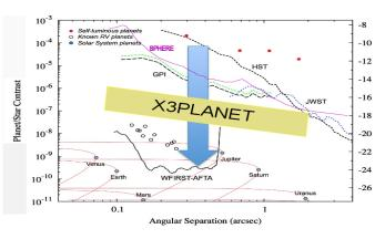
The above figure shows the capability of the 2.4 m WFIRST-AFTA space facility; based on figure from the WFIRST-AFTA SDT Interim Report, by D. Spergel et N. Gehrels. On the figure was added the typical SPHERE on-sky performances (in pink) together with (yellow box) the contrast/parameter range of the proposed X3PLANET facility
