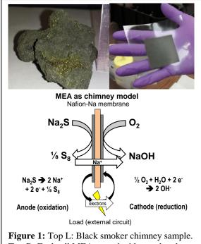
Top R: Fuel cell MEA coated with powdered geocatalyst on both sides. Lower: Model of hydrothermal chimney as fuel cell experiment.
