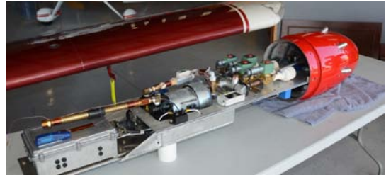
Fig. 2. The DART internal subsystems. Six external scoops can be seen on the nosecone, and the filter housings hold 47 mm filters forward of the green solenoid valves.
