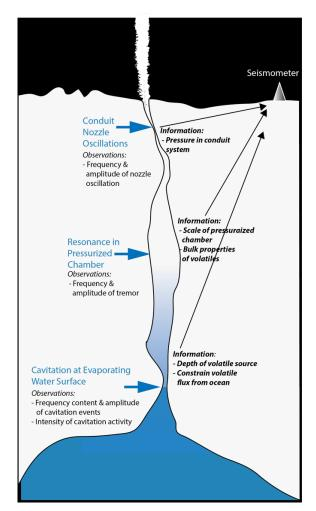
**Figure 1:** Inspired by Spencer and Nimmo [4], potential seismic sources (blue text) and how they might be used to constrain the physical properties and parameters of a cryovalcano system. The hypothesized seismic sources of cavitation, chamber resonance, and nozzle oscillations are based on terrestrial analogues of geysers, volcanoes and volcanic nozzles respectively.
