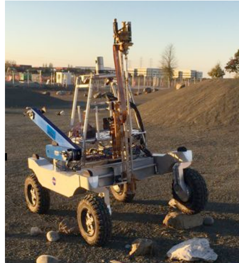
Fig. 1. Initial integration in December 2016 of the ARADS biomarker-search test vehicle, with drill, sample transfer arm, on the KREX2 rover.
