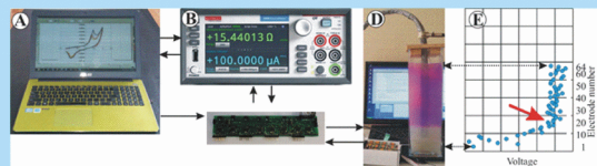
Fig. 4. Measurement setup of a working SPEAR instrument: (A) Computer controlling the measuring instrument and the multichannel selector. (B) Dual channel potentiostat. (C) Multichannel selector (analog multiplexer). (D) Probe with 64 working electrodes, one reference electrode and one counter electrode. (E) Vertical redox potential profile produced with all 64 electrodes.
