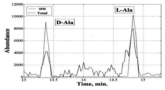
Section of the total ion chromatogram of amino acids (N-trifluoroacetyl, isopropyl esters) extracted from the impact sample, with the retention times for D-Ala and L-Ala at 13.3 s and 14.7 s, respectively, derived from SIM mode. Comparison of chromatograms in SIM mode and total ion mode to verify the retention times for D-Ala and L-Ala. In SIM mode the mass 140 amu was used for D-Ala and L-Ala.
