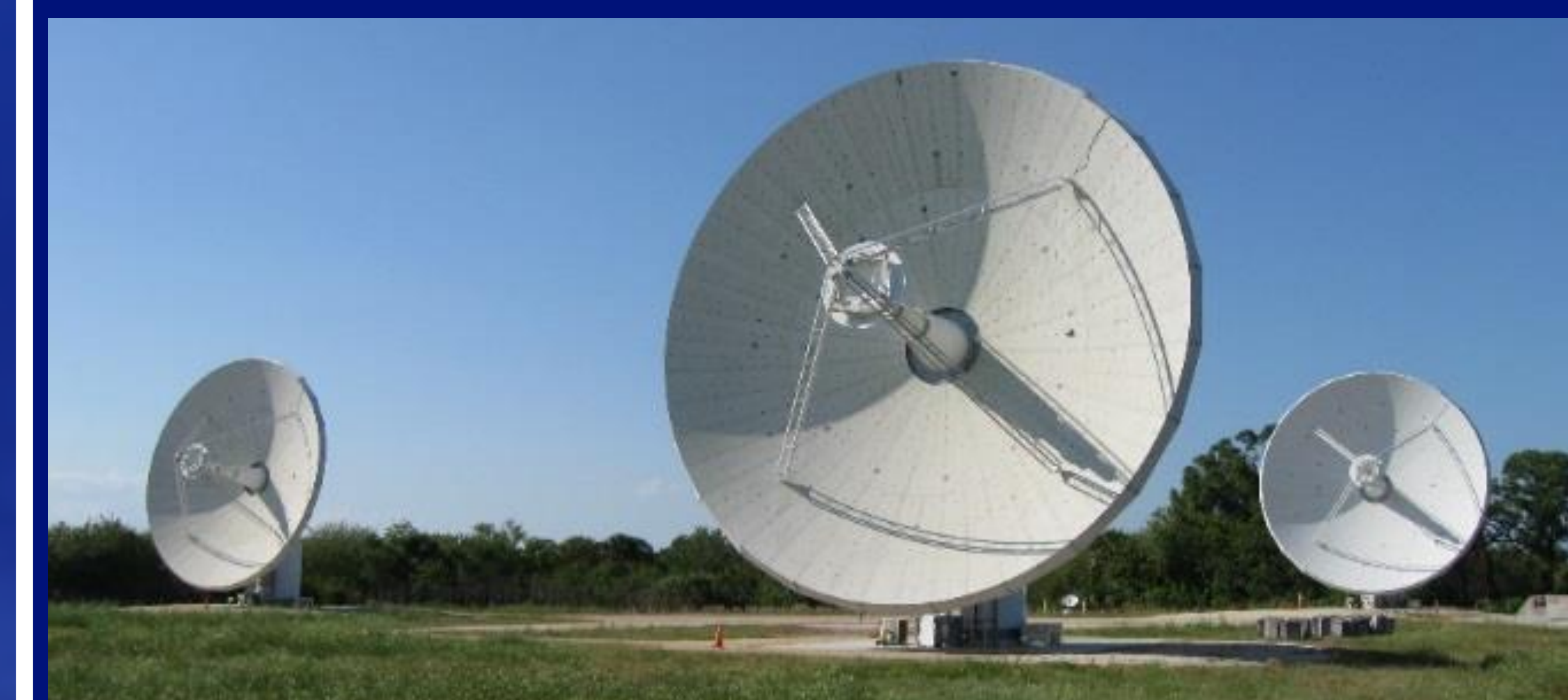
KaBOOM Ka-band three-element (12-m) phased array testbed
